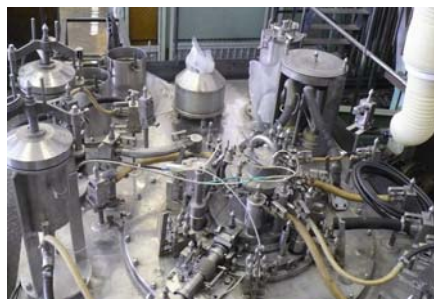
Chlorator-electrolyzer under testing
