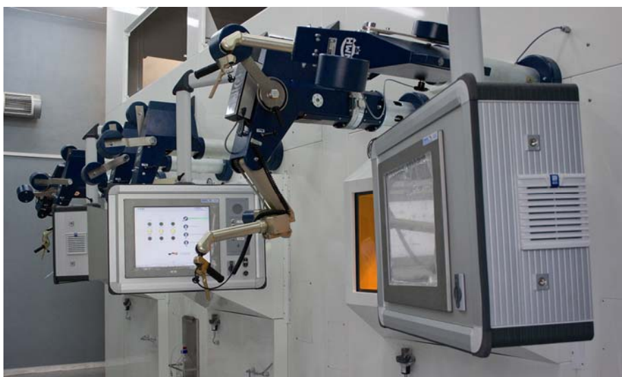
Shielded boxes for irradiated targets reprocessing
